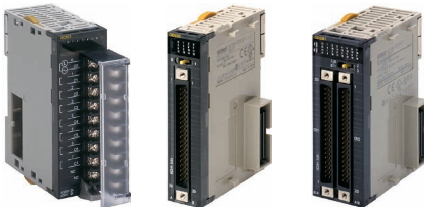
Figure 2-10 16, 32, and 64 point I/O modules.
