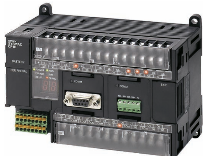
Figure 14-43 Omron PLC with Modbus-RTU network communication capabilities.
