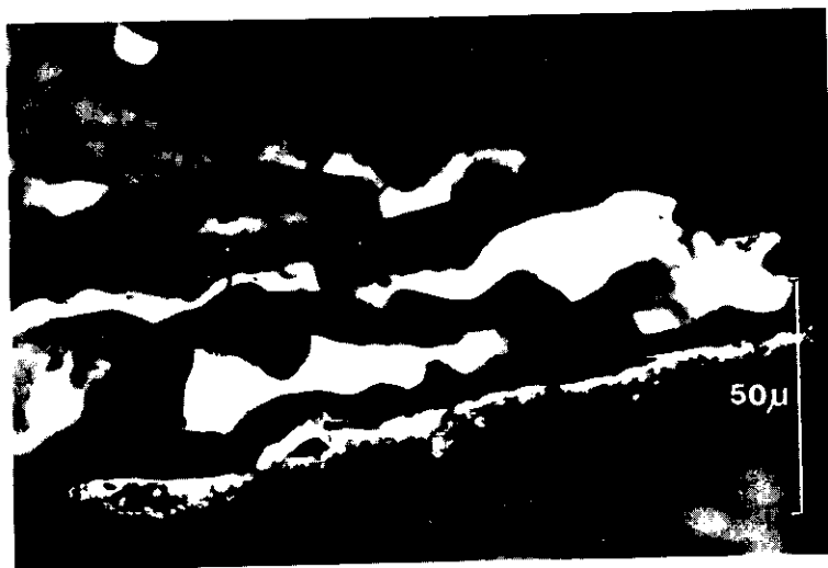
Fig. V.1.2. An altered inertinite particle, showing darkening due to weathering (oxidation). Reflected light, oil immersion. (Photo Hagemann)
