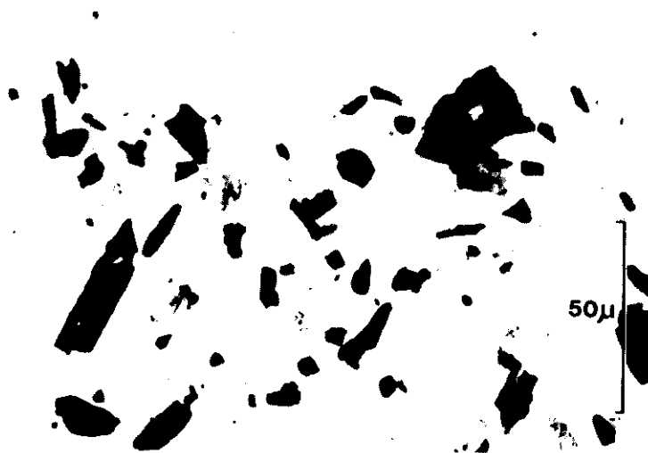
Fig. V.1.4. A kerogen in transmitted light: small angular dark objects are vitrinitic plant particles. The grey transparent object in upper right corner is a fragment of cuticle; the long dark perforated object in lower left corner is fusinite. Kerogen concentrate of Upper Liassic shale (Pliensbachian), Luxembourg. Transmitted light. (Photo Hagemann)
