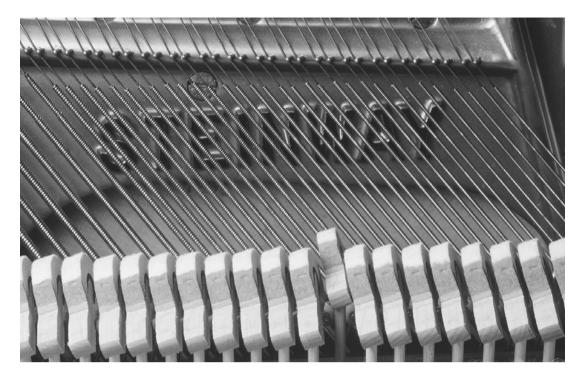
PIAND STRINGS GENERATE SOUND AS THEY ARE SET INTO VIBRATION BY THE HAMMERS. THE HAMMERS, IN TURN, ARE ATTACHED TO THE BLACK-AND-WHITE KEYS ON THE OUTSIDE OF THE PIAND. (Photograph by Bob Krist/Corbis. Reproduced by permission.)
