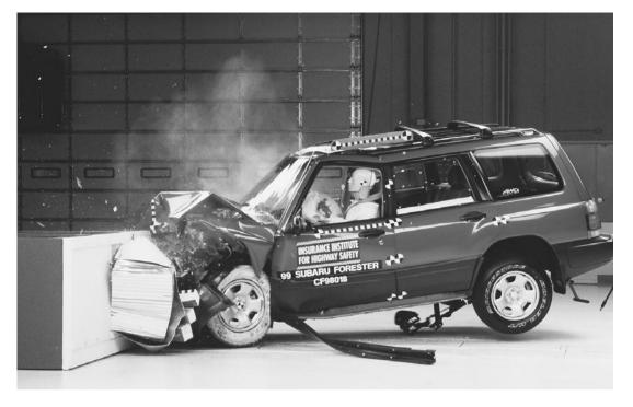
WHEN A VEHICLE HITS A WALL, AS SHOWN HERE IN A GRASH TEST, ITS MOTION WILL BE STOPPED, AND QUITE ABRUPT-LY. BUT THOUGH ITS MOTION HAS STOPPED, IN THE SPLIT SECONDS AFTER THE GRASH IT IS STILL RESPONDING TO INERTIA: RATHER THAN BOUNCING OFF THE BRICK WALL, IT WILL CONTINUE PLOWING INTO IT. (Photograph by Tim Wright/Corbis. Reproduced by permission.)
