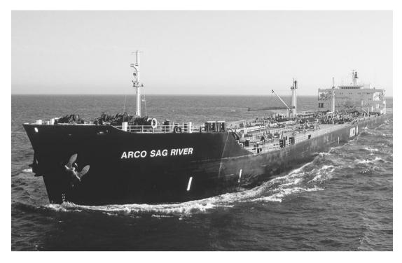
How does a gigantic steel ship, such as the supertanker pictured here, stay afloat, even though it has a weight density far greater than the water below it? The answer lies in its curved hull, which contains a large amount of open space and allows the ship to spread its average density to a lower level than the water. (*Photograph by Vince Streano/Corbis. Reproduced by permission.*)
