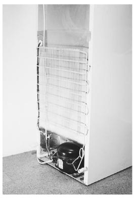
A REFRIGERATOR IS A TYPE OF REVERSE HEAT ENGINE THAT USES A COMPRESSOR, LIKE THE ONE SHOWN AT THE BACK OF THIS REFRIGERATOR, TO COOL THE REFRIGERATOR'S INTERIOR. (Ecoscene/Corbis. Reproduced by permission.)
