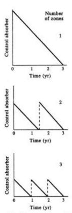
Fig. 19.7 Reactor operation with different numbers of fuel zones. The initial control absorber varies inversely with the number of regions.
