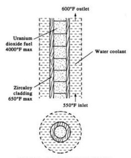
Fig. 12.4 Reactor channel heat removal.
