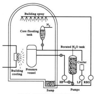
Fig. 19.9 Emergency core cooling system.
