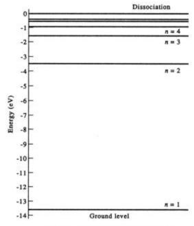
Fig. 2.4 Energy levels in hydrogen atom.
