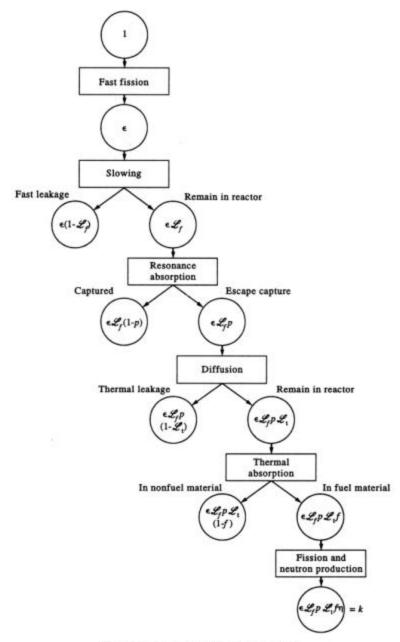
Fig. 11.4 Neutron cycle in thermal reactor.
