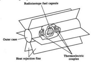
Fig. 20.2 Isotopic electrical power generator. (SNAP-27 used in Apollo-12 mission.)
