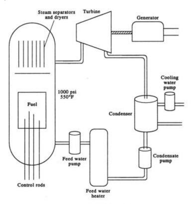
Fig. 12.8 BWR system flow diagram.
