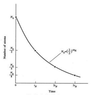
Fig. 3.1 Radioactive decay.
