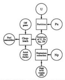
Fig. 22.5 Simplified flow chart of nuclear fuel reprocessing.
