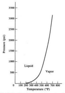
Fig. 12.5 Relationship of pressure and temperature for water.
