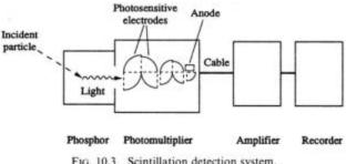
Fig. 10.3 Scintillation detection system.
