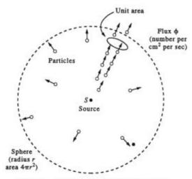
Fig. 21.1 Inverse square spreading of radiation.
