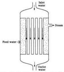
Fig. 12.6 Heat exchanger or steam generator.
