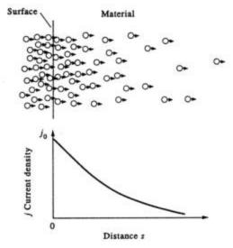
Fig. 4.4 Neutron penetration and attenuation.
