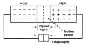
Fig. 10.5 Solid-state n-p junction detector.
