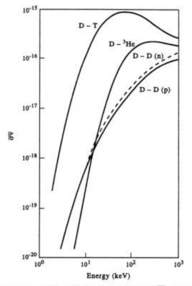
Fig. 14.1 Reaction rates for fusion reactions. The quantity  $\sigma v$ , the average over a Maxwellian distribution of cross section times speed, when multiplied by particle densities gives the fusion rate per unit volume.
