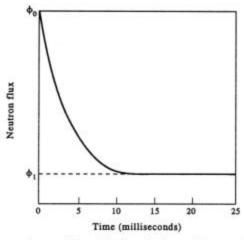
Fig. 19.6 Neutron flux variation with time in the rod-drop method of measuring reactivity.
