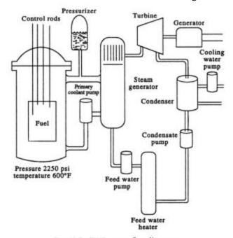
Fig. 12.7 PWR system flow diagram.
