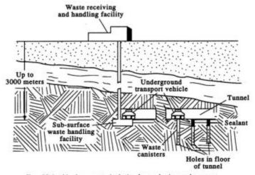
Fig. 22.6 Nuclear waste isolation by geologic emplacement.
