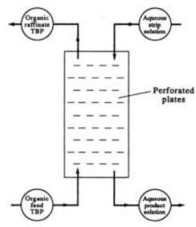
Fig. 22.4 Solvent extraction by the Purex method.
