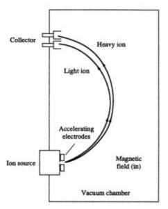
Fig. 9.1 Mass spectrograph.
