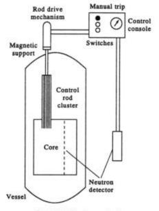
Fig. 19.4 Reactor control.
