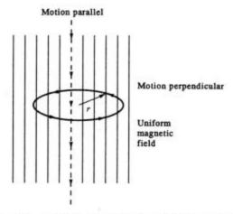
Fig. 8.2 Electric charge motion in uniform magnetic field.
