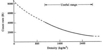
Fig. 17.7 Direct-transmission radiation gauge to measure soil density. (Courtesy of Troxler Electronic Laboratories, Inc.)
