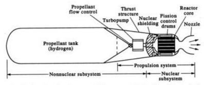
Fig. 20.4 Nuclear-thermal rocket system. Hydrogen stored in liquid form is heated in the solid core and expelled as propellant. (Courtesy Gary Bennett).
