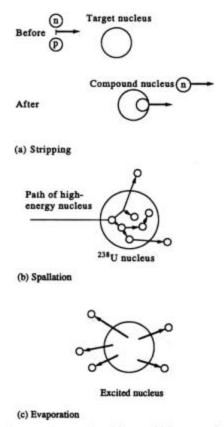
Fig. 8.10 Nuclear reactions produced by very high energy charged particles.
