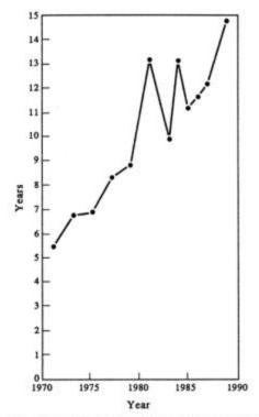
Fig. 24.2 Construction times for nuclear power plants. Adapted from DOE/EIA-0439(84).
