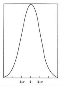
Fig. 10.6 Gaussian distribution. The area between the limits  $x \pm \sigma$  is 68% of the total.
