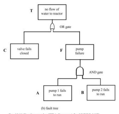
Fig. 19.11 Simple example of PRA diagrams (after NUREG-0492)
