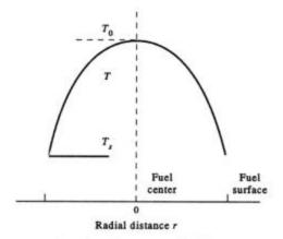
Fig. 12.1 Temperature in fuel.
