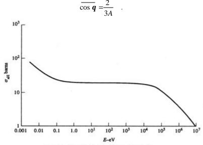
Fig. 4.7 Scattering cross section for hydrogen.
