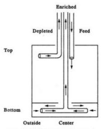
Fig. 9.6(b) Gas streams in centrifuge.
