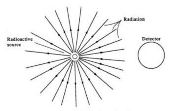
Fig. 3.2 Measurement of radiation from radioactive source.
