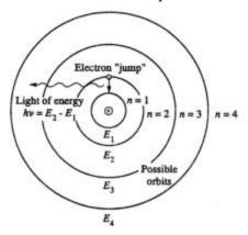
Fig. 2.3 Electron orbits in hydrogen (Bohr theory).
