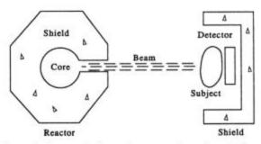
Fig. 17.6 Schematic diagram of a thermal neutron radiography unit. Source can be an accelerator, a reactor, or a radioisotope.
