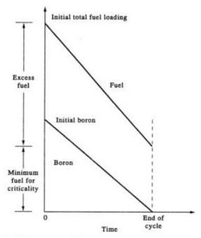
Fig. 11.6 Reactor control during fuel consumption in power reactor.
