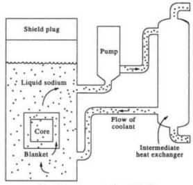
Fig. 13.1 Loop system for LMFBR.
