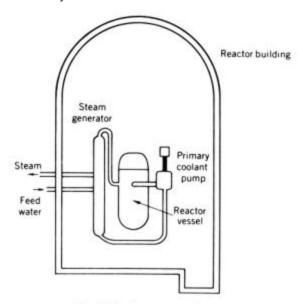
Fig. 19.8 Reactor containment.
