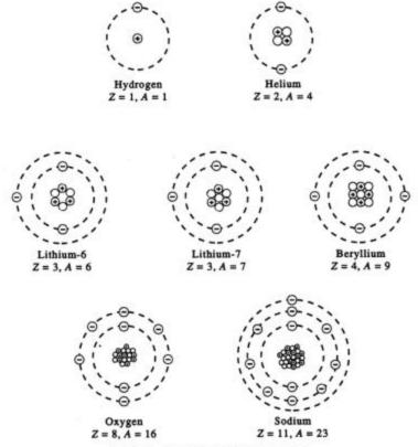
Fig. 2.7 Atomic and nuclear structure.
