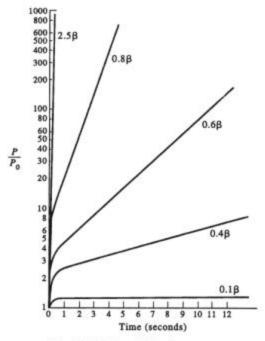
Fig. 19.2 Effect of delayed neutrons.
