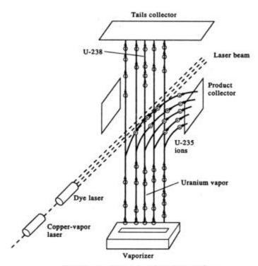
Fig. 9.8 Atomic vapor laser isotopic separation.
