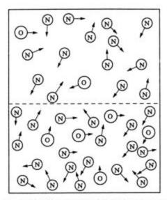
Fig. 9.2 Gaseous diffusion separation of nitrogen and oxygen.
