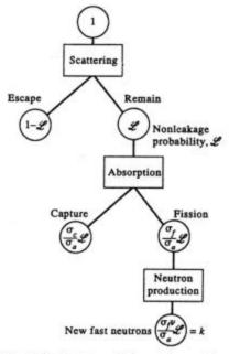
Fig. 11.3 Neutron cycle in metal assembly.
