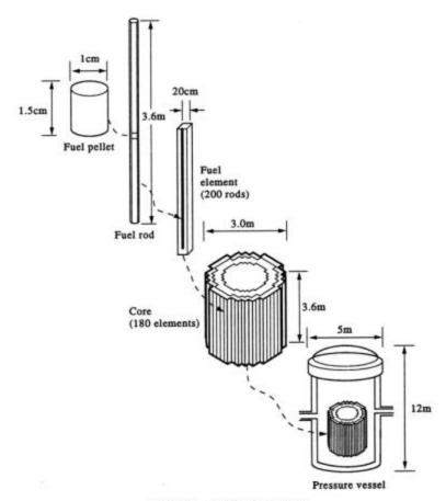
Fig. 11.5 Reactor construction.
