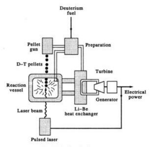
Fig. 14.6 Laser-fusion reactor.
