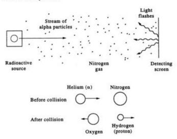
Fig. 4.1 Transmutation by nuclear reaction.
