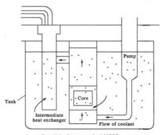
Fig. 13.2 Pot system for LMFBR.
