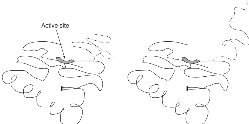
FIGURE 1.5. Schematic drawing showing the use of a temperature sensitive polymer to control access to the active sites of an enzyme. Access is denied when the polymer (dotted line) is in the crystalline state (left), and allowed when the polymer is in the flexible state (right).
