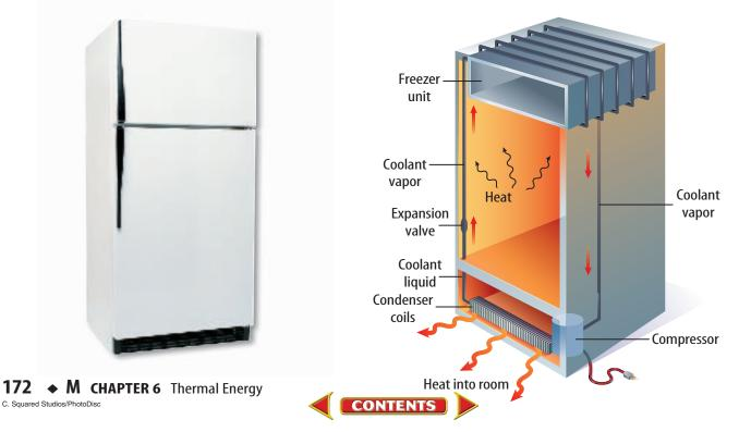
**Air Conditioners** Most air conditioners cool in the same way that a refrigerator does. You've probably seen airconditioning units outside of many houses. As in a refrigerator, thermal energy from inside the house is absorbed by the coolant within pipes inside the air conditioner. The coolant then is compressed by a compressor, and becomes warmer. The warmed coolant travels through pipes that are exposed to the outside air. Here the thermal energy is transferred to the outside air.
