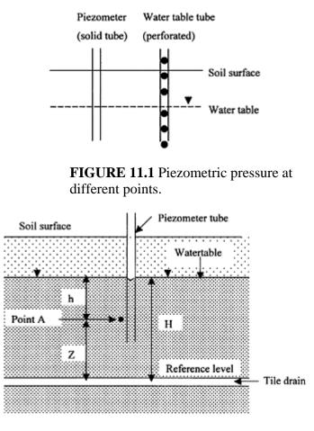
**FIGURE 11.2** A piezometer tube showing the soil water pressure below the water table. At the reference point A, the pressure potential equals  $h (\phi_p = h \text{ cm})$ , gravitational potential *z*, and the total potential H=(h+Z).
