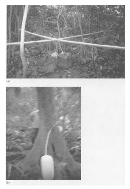
**FIGURE 9.14** (a) Spider gauge to measure through-fall and (b) stem flow.
