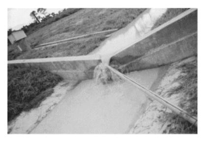
**FIGURE 9.17** A wier with a slot-pipe to collect runoff sample.
