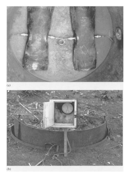
**FIGURE 9.23** (a) A hydraulic weighting device may involve water-filled pillows placed beneath the lysimeter, and (b) connected to a pressure gauge.
