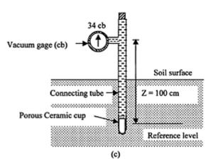
FIGURE 11.3 Different types of tensiometers: (a) a water manometer connected to a ceramic cup installed in soil at the designated depth,  $\Phi_m$  equals -h; (b) a mercury manometer connected to a ceramic cup installed in soil at the desired depth,  $\Phi_m = -Z_{Hg} \times 13.6 + Z$ ; and (c) a vaccum gauge tensiometer,  $\Phi_m = -34 \times 10$ cm+100 cm=-240 cm.
