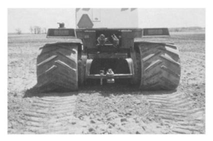
**FIGURE 7.14** Similar to dual tires, wide tires can also distribute the load over a large area. Nonetheless, the
