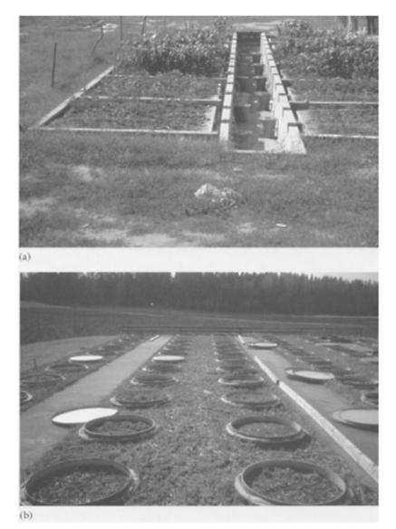
**FIGURE 9.24** A battery of drainage lysimeter (a) with a trench to collect seepage; (b) an underground weighing and seepage collection facility.
