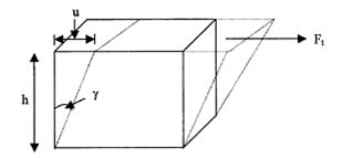
**FIGURE 7.1** Shear strain exemplified by angular deformation.
