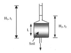
**FIGURE 12.6** Schematic of falling head method for *K*<sub>s</sub> measurement.
