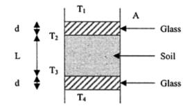
**FIGURE 17.8** Apparatus for measurement of thermal conductivity under steady state.
