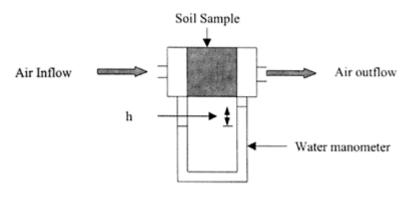
FIGURE 18.4 Schematic of the apparatus of measure air permeability  $(k_a)$ .
