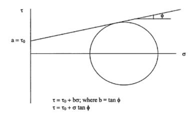
**FIGURE 7.2** The functional relationship between shearing stress ( $\tau$ ) and normal stress ( $\sigma$ ) is given by Mohr's circle (*a* or  $\tau_0$  is the intercept and constant *b* is the tangent of angle  $\phi$
