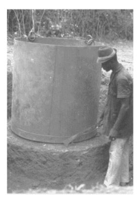
**FIGURE 9.20** Installation of a circular monoleith lysimeter.
