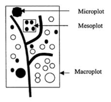
**FIGURE 19.6** The schematic of micro-, meso-, and macroplots for studying soil erosion by water. (Modified from Poesen et al., 1994.)
