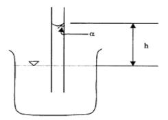
**FIGURE 5.2** Capillary rise of water to height *h* in a glass tube.
