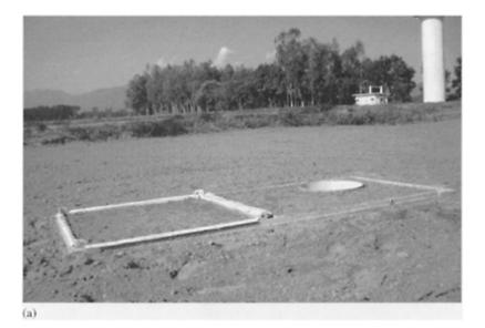
**FIGURE 9.19** A square filled in lysimeter (a) method and (b) with removable cover.
