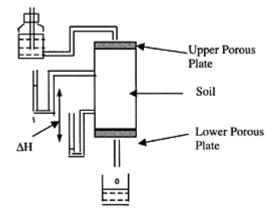
FIGURE 13.7 Schematic of a system for the measurement of unsaturated hydraulic conductivity under steady state condition.
