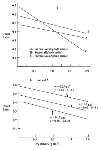
**FIGURE 7.11** The effect of (a) soil texture, and (b) gravimetric soil moisture content on density probe calibration. (Redrawn from Lal, 1974.)
