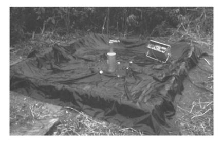
**FIGURE 10.9** A plastic covered plot is used to assess field water capacity using a neutron moisture meter. After saturing the plot with sufficient water, the plastic cover was used to prevent evaporation. (Ibadan, Nigeria, 1971)
