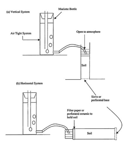
**FIGURE 14.12** Measurement of infiltration in soil columns using a Marriotte bottle technique.
