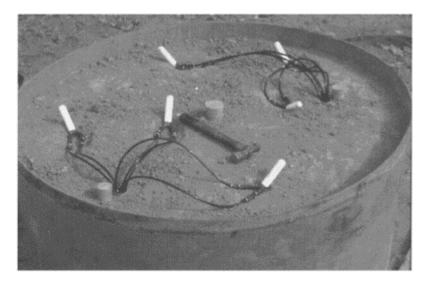
**FIGURE 9.21** A suction cup and neutron probe access tube are installed at the base.
