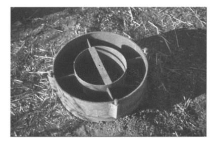
**FIGURE 14.13** A double ring infiltrometer. The outer ring is 30–50 cm in diameter and the inner ring 20– 30 cm. Both rings are 20 to 30 cm high.
