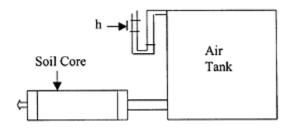
**FIGURE 18.5** Schematic of an air permeability apparatus on soil cores for a transient method.
