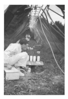
**FIGURE 14.15** Rainfall simulators are commonly used to assess infiltration rate under nonponded condition.
