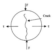
**FIGURE 7.3** Schematic of loading (*F*) of an aggregate at poles and the resultant tensile stress ( $\tau$ ) at right angles to *F* and development of a crack as  $\tau$  approaches tensile strength (*S<sub>T</sub>*) of soil.
