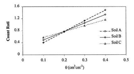
**FIGURE 19.4** Effect of soil texture on neutron probe calibration for moisture content determinations for soil A (0.8% gravel, 41% sand, and 15.2% clay content), soil B (59.7%, 27.1%, 7.3%), and soil C (8.2%, 16.3%, 63.9%). (Recalculated and drawn from Lal, 1974.)
