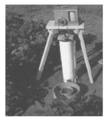
**FIGURE 14.14** The change in height of water in a column used to assess infiltration can also be measured using a water stage recorder.
