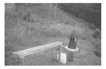
**FIGURE 9.11** Recording and non-recording rain gauges.
