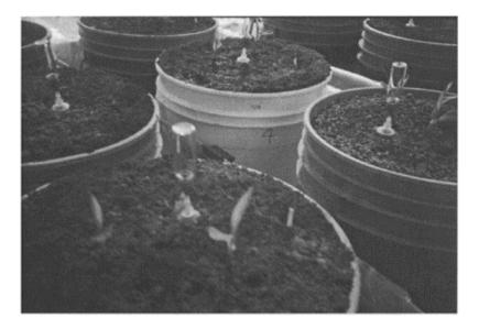
**FIGURE 18.**2 Soil air diffusion tube installed in a greenhouse water table management experiment. Similar
