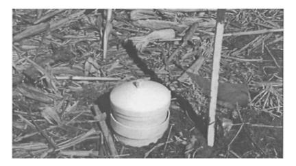
**FIGURE 18.3** A static chamber is used under field conditions to assess the gaseous emission over a short period of 10 to 15 minutes. (Waterman Farm, Columbus, OH, 1998.) surface and can be expressed as follows:
