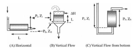
**FIGURE 12.5** Schematic of apparatus for saturated hydraulic conductivity: (A) horizontal, (B) vertical flow, (C) vertical flow from bottom.
