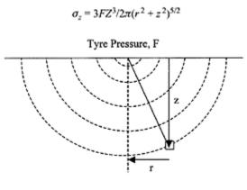
**FIGURE 7.9** Pressure distribution under a tire per the Boussinesq equation.
