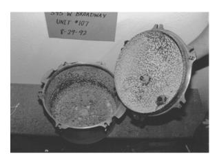
Figure 9.6 Interior of pressure cooker.
