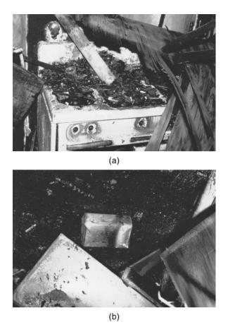
**Figure 2.2** Fire from methanol evaporating on a gas stove. (a) Gas stove fire point of origin. (b) Burned methanol container.
