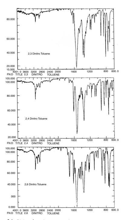
Figure 5.4 Dinitrotoluene isomer comparison.
