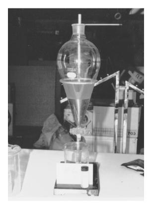
Figure 9.11 Conventional separatory funnel containing a two-phase liquid.
