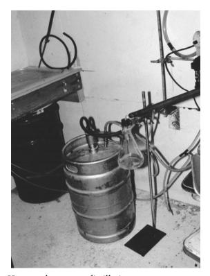
Figure 9.10 Homemade vacuum distillation apparatus.
