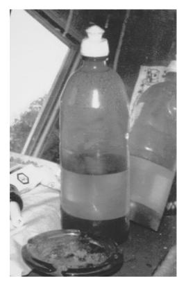
Figure 9.12 Plastic soda bottle used as a separatory funnel.
