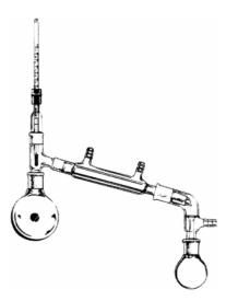
**Figure 1.6** Simple distillation apparatus.
