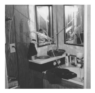
Figure 9.9 Inverted condensing column on a distillation apparatus.
