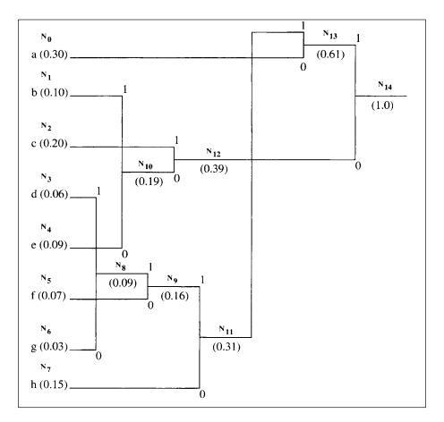
Fig. 15.2 Huffman tree construction for Example 1.
