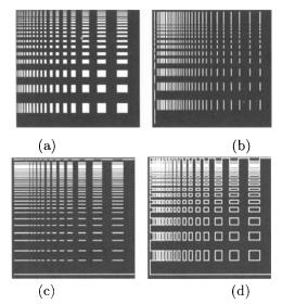
Fig.~7.3~ (a) Input image, (b) vertical edges, (c) horizontal edges, (d) edge image along both directions.
