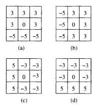
Fig. 7.8 Kirsch masks to compute gradients in four directions.
