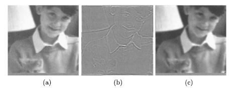
Fig. 6.4 (a) Input image, (b) High-passed filtered, (c) Low-pass filtered output images.
