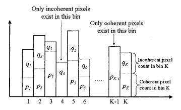
Fig. 11.2 Partitioning the color histogram with coherence and noncoherence pixel counts.
