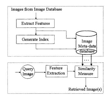
Fig. 11.1 Architecture of a content-based image retrieval system.
