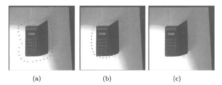
$Fig.\ 9.3~$  Results of active contour modelling by SNAKE - (a) original Image, (b) contour after 10 iterations, (c) final contour.
