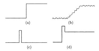
Fig. 7.2 Different types of edges: (a) step, (b) ramp, (c) line, (d) step-line.
