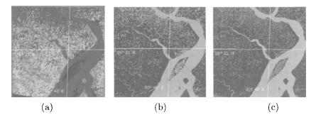
*Fig. 13.2* Satellite Image (a) original, (b) segmented by multilayered perceptron (error backpropagation), (c) segmented by Fuzzy self-organizing feature map.
