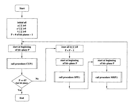
Fig. 18.6 Top-level flowchart of fractional bit-plane coder for P > 0.
