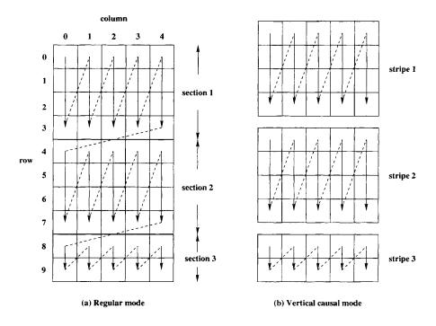
Fig. 18.1 Scan pattern with a  $5\times10$  code-block: (a) regular mode; (b) vertical causal mode.
