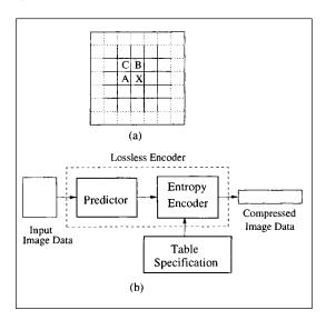
$Fig. \ 16.1$  (a) Three-pixel prediction neighborhood, (b) encoder diagram in lossless mode.
