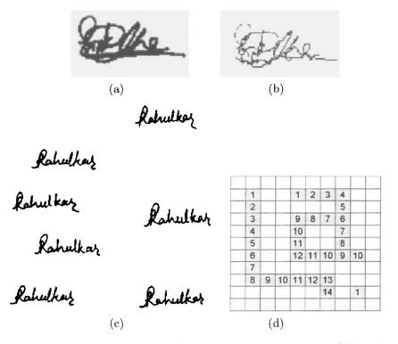
Fig. 12.3 Signature Image (a) Original (b) Thinned version of the original (c) Samples of original and forged signatures (d) example of waterfilling
