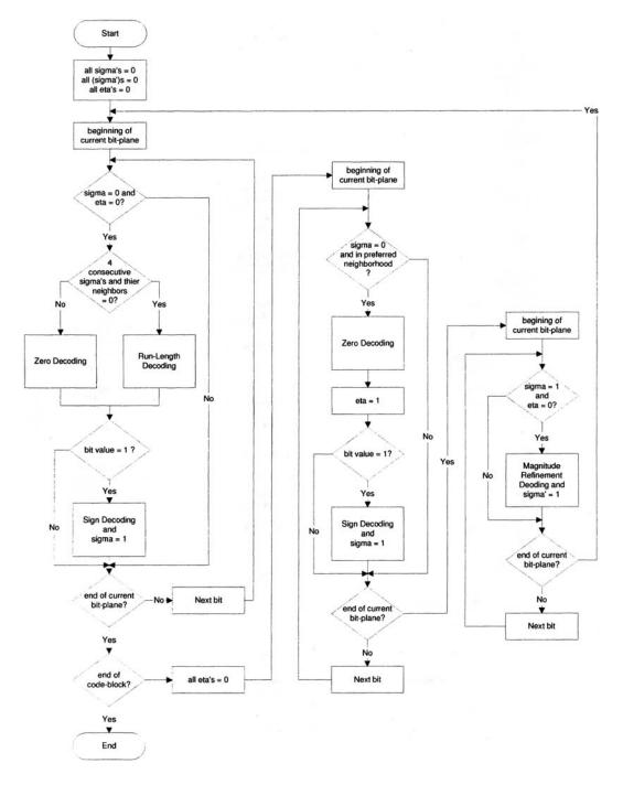
Fig. 18.8 Flowchart of fractional bit-plane decoder for P > 0.
