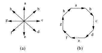
Fig. 8.4 (a) Example of a Freeman chain code (b) Freeman chain code of an octagon.
