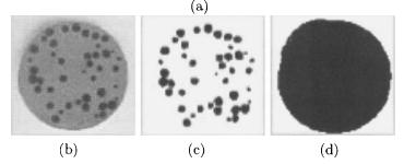
Fig. 7.15 Multilevel Image thresholding: (a) Multimodal Histogram, (b) input image, (c) segmented foreground objects, (d) segmented background.
