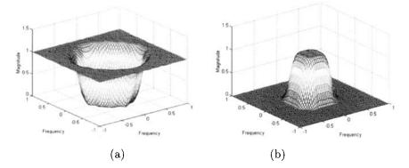
Fig. 6.3 Two-dimensional filter response (a) high-pass, (b) low-pass.
