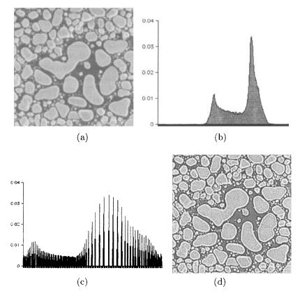
Fig. 6.1 Histogram equalization results: (a) original image, (b) histogram of the image, (c) equalized histogram (d) enhanced image.
