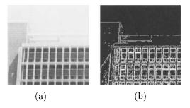
Fig. 7.9 (a) Original image, (b) edge image by Canny's edge detector.
