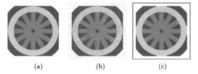
Fig. 6.2 Result of median filtering: (a) original image, (b) salt and pepper noisy image, (c) result of median filtering.
