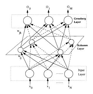
Fig. 8.8 Architecture of a Counterpropagation Neural Network.
