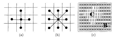
Fig. 2.9 Examples of (a) 4-connected pixels, (b) 8-connected pixels, and (c) connected component and background.
