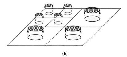
Fig. 17.5 (a) ROI mask; (b) scaling of ROI coefficients.
