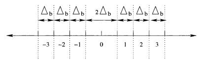
Fig. 17.3 Dead-zone quantization about the origin.
