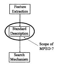
Fig. 11.6 Scope of the MPEG7 standard.
