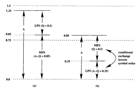
Fig. 15.5 Subinterval assignment in QM-coder, (a) without conditional exchange and (b) with conditional exchange.
