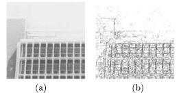
Fig. 7.12 (a) Original image, (b) edge image by Laplacian edge detector.
