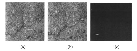
Fig. 13.3 Change detection from repeat pass SAR image: (a) original, (b) repeat pass of the original after a time interval, (c) changes in them.
