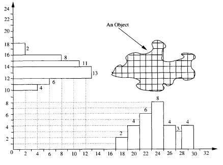
Fig. 2.10 Histogram of a binary object along horizontal and vertical axes.
