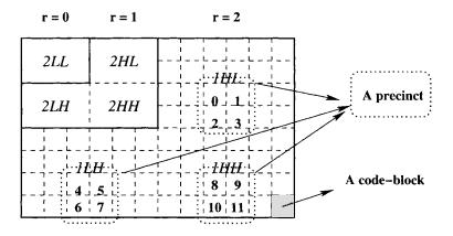
Fig. 18.9 A precinct from a two-level DWT with three resolutions.
