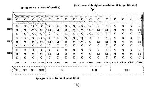
Fig. 18.10 (a) A two-level DWT with 16 code-blocks, (b) bitstream formations. (Note: The letters S, M, and C in (b) stand for the bitstream generated during significance propagation pass, magnitude refinement pass, and cleanup pass, respectively.)
