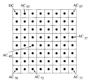
Fig. 16.4 DC and AC components of the transformed block.
