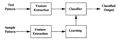
Fig. 8.1 Block diagram of a decision theoretic pattern classifier.
