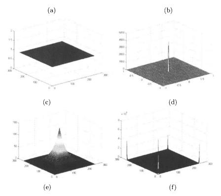
*Fig. 4.1* Examples: (a) square image, (b) DFT magnitude of the square image, (c) two-dimensional DC signal, (d) DFT magnitude of the DC signal, (e) two-dimensional exponential function, (f) DFT magnitude of the exponential function.
