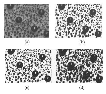
$\it Fig.~7.16~$  Comparison of thresholding techniques: (a) original image, (b) Otsu, (c) Kapoor, and (d) Renyi's Entropy.
