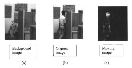
Fig. 14.1 Results of background modeling and segmentation of a moving human figure: (a) modelled background, (b) an input frame, (c) segmented human object.
