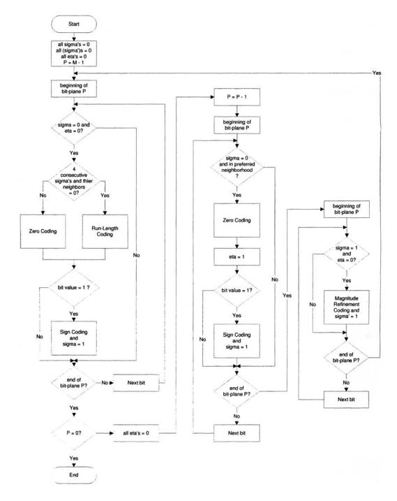
Fig. 18.7 Flowchart of fractional bit-plane encoder for P>0 .
