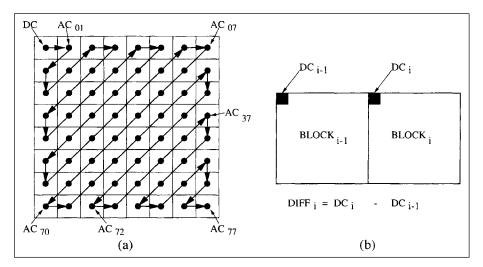
Fig. 16.5 (a) Zig-zag ordering of AC coefficients; (b) differential coding of DC.
