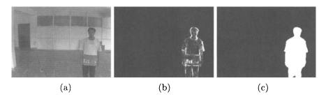
Fig. 7.18 (a) An original image, (b) interframe difference image, (c) segmented human object.
