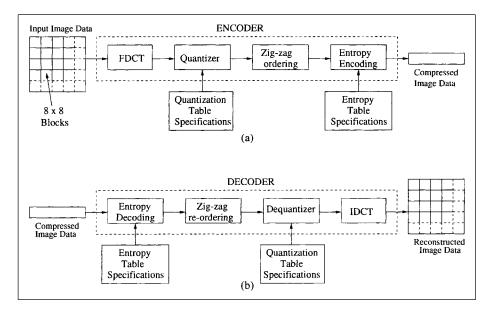
Fig. 16.3 Baseline JPEG: (a) compression, (b) decompression.
