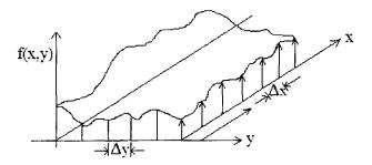
Fig. 2.4 Two-dimensional sampling array.
