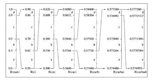
Fig. 15.3 Arithmetic coding technique: an example.
