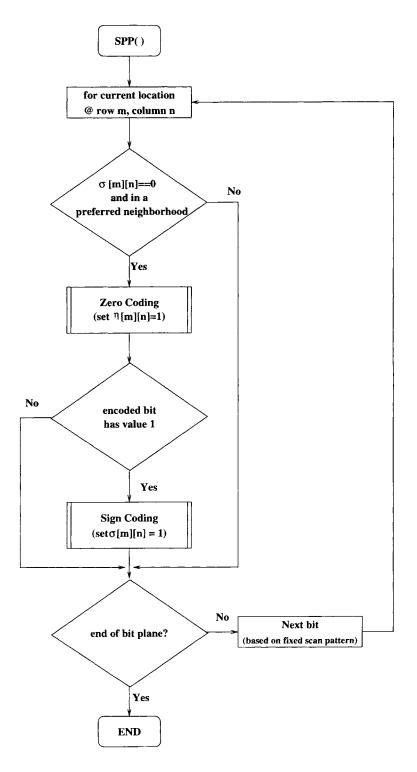
Fig. 18.4 Flowchart of significance propagation pass.
