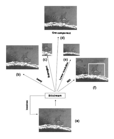
Fig. 17.1 Example of capabilities of JPEG2000 technology.
