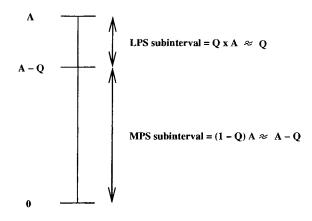
Fig. 15.4 Subinterval assignment in QM-coder.
