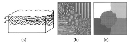
Fig. 9.2 (a) Covering blanket to compute fractal dimension, (b) A multi-textured image, (c) segmented image using fractal dimension
