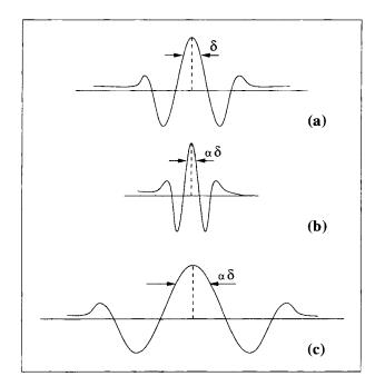
Fig. 5.1 (a) A mother wavelet  $\psi(t)$ , (b)  $\psi(t/\alpha)$ :  $0 < \alpha < 1$ , (c)  $\psi(t/\alpha)$ :  $\alpha > 1$ .
