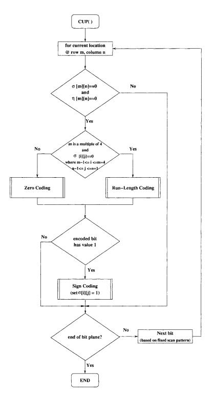
Fig. 18.3 Flowchart of cleanup pass.
