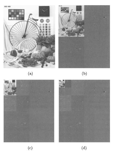
Fig. 5.5 (a) Original BIKE image and subbands; (b) after level 1, (c) after level 2, (d) after level 3 decomposition.
