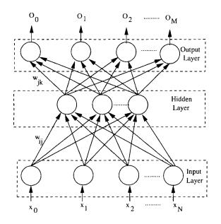
Fig. 8.6 Architecture of a Backpropagation Neural Network.
