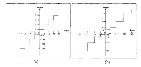
Fig. 2.7 Two-dimensional (a) uniform quantization (b) nonuniform quantization.
