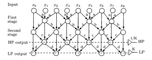
Fig. 5.8 Data dependency diagram with four lifting factors.
