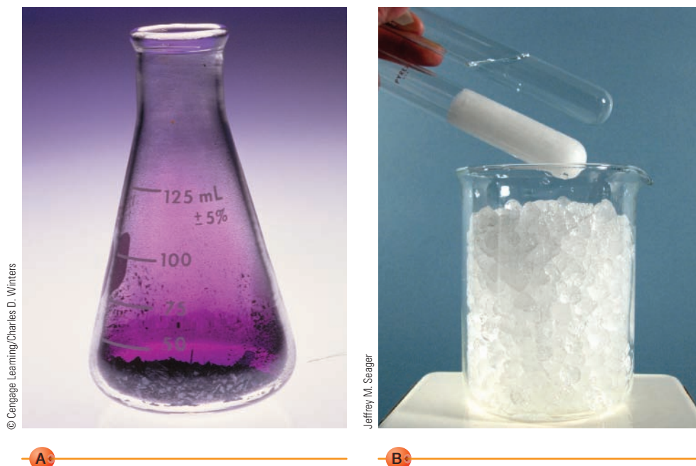
Figure 1.2 Examples of physical change: Solid iodine becomes gaseous iodine when heated A ; liquid benzene becomes solid benzene when cooled B .
