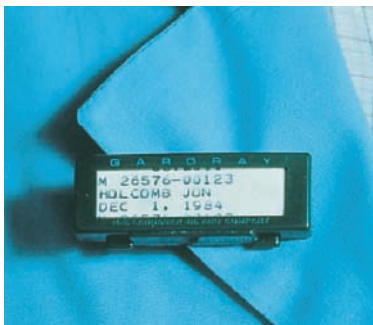
Figure 10.4 Film badges provide a convenient way to monitor the total amount of radiation received during a specific time period.
