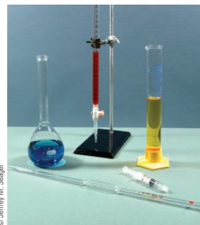
Figure 1.13 Glassware for measuring volumes of liquids. Clockwise from top center: buret, graduated cylinder, syringe, pipet, and volumetric flask.
