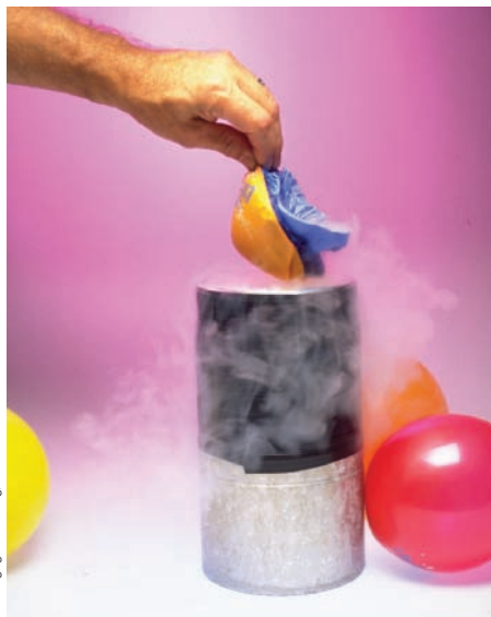
Figure 6.6 A balloon collapses when the gas it contains is cooled in liquid nitrogen (temperature = -196^{\circ}\text{C} , or 77\text{ K} ). Assume the inflated yellow balloon had a volume of 4.0\text{ L} at room temperature ( 25^{\circ}\text{C} ) and the prevailing pressure. Assume the pressure remained constant and calculate the volume of the gas in the balloon at the temperature of liquid nitrogen.
