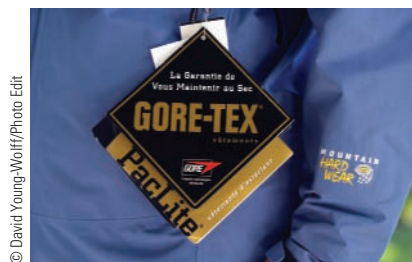
Figure 12.6 Gore-Tex® is a thin, membranous material made by stretching Teflon fibers. Fabrics layered with Gore-Tex repel wind and rain but allow body perspiration to escape, making it an excellent fabric for sportswear.
