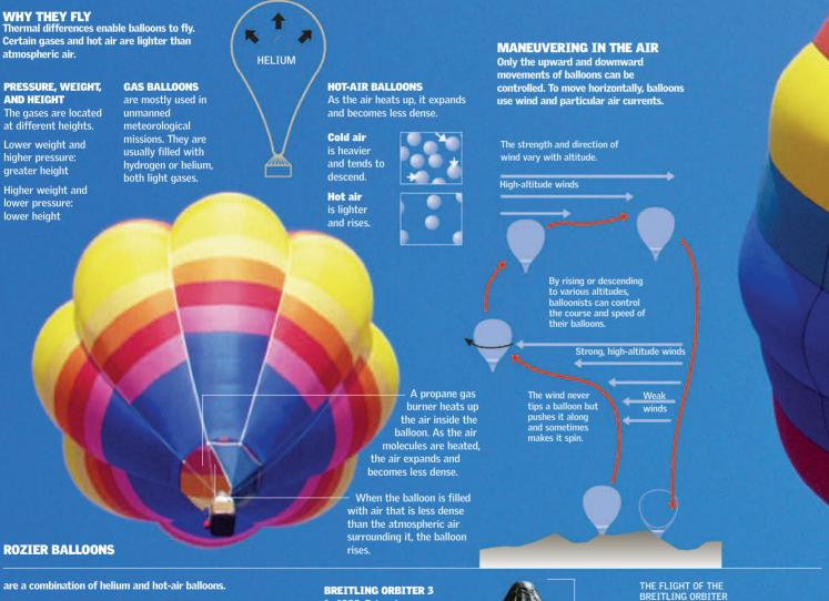
The balloonist can change altitude by controlling air temperature.
