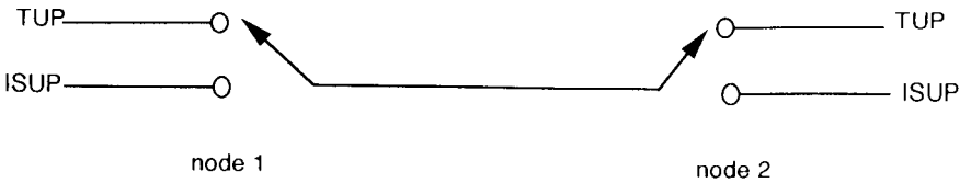
Figure 8.14 User data transport protocol between nodes using MTP layer.
