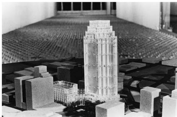
■ FIGURE 7.1 Model of the National Bank of Commerce, San Antonio, Texas, for measurement of peak, rms, and mean pressure distributions. The model is located in a long-test-section, meteorological wind tunnel. (Photograph courtesy of Cermak Peterka Petersen, Inc.)
