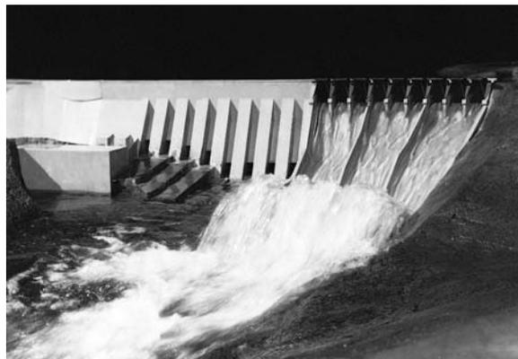
■ **FIGURE 7.2** A scale hydraulic model (1:197) of the Guri Dam in Venezuela, which is used to simulate the characteristics of the flow over and below the spillway and the erosion below the spillway. (Photograph courtesy of St. Anthony Falls Laboratory.)
