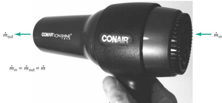
■ FIGURE 5.7 One inlet, one outlet flow.
