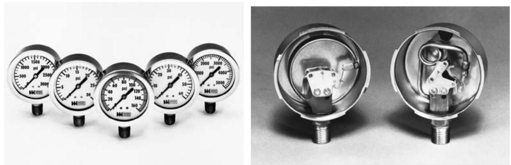
**FIGURE 2.10** (a) Liquid-filled Bourdon pressure gages for various pressure ranges. (b) Internal elements of Bourdon gages. The “C-shaped” Bourdon tube is shown on the left, and the “coiled spring” Bourdon tube for high pressures of 1000 psi and above is shown on the right. (Photographs courtesy of Weiss Instruments, Inc.)
